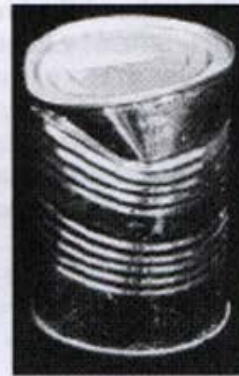
Sharp dent or dent on seam
